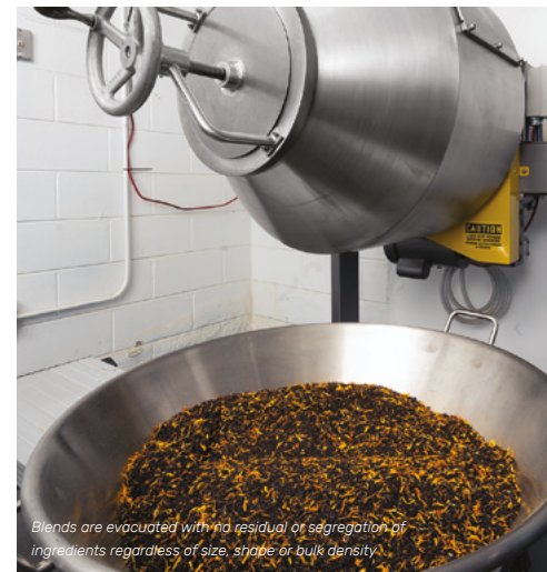
The mixer's tumble-turn-cut-fold action achieves uniformity in three minutes with no product degradation
