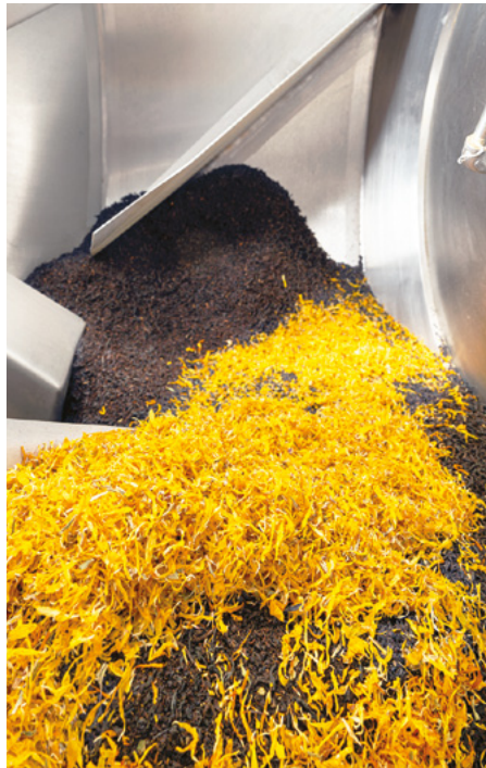
The mixer's tumble-turn-cut-fold action achieves uniformity in three minutes with no product degradation
