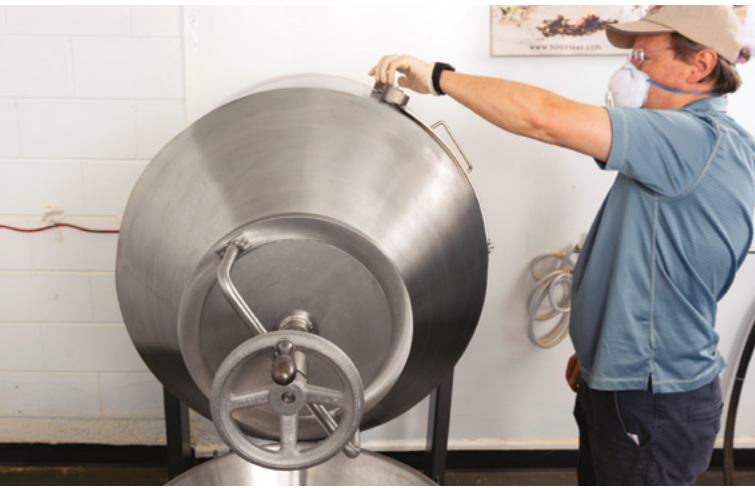
Blending in-house: Biron Teas' 85 litre-capacity Rotary Batch Mini Mixer blends teas with or without liquid additions in three minutes with no shear or damage to delicate ingredients
